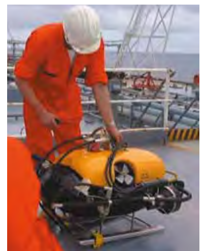
The Seaeeye 600 DT being prepared for an inspection.
