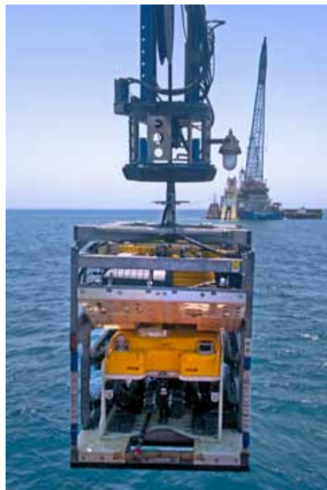
A Cougar XT ROV was deployed by SMIT Subsea for pipeline touchdown monitoring for Kito Enterprises.
