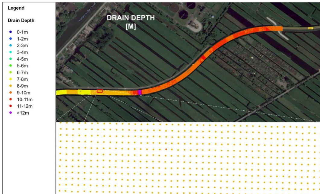
Figure 7. GIS overview of PVD installation depth and installation accuracy.
