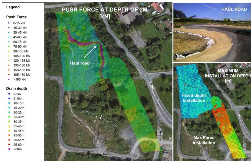
Figure 6. GIS compilation of the logger data showing the push for at 2m installation depth and the maximum installation depth over the project area.
