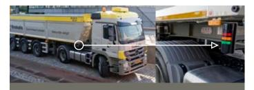
Boskalis BV has developed a new system to prevent trucks from becoming overloaded. Three lights are installed on the side of the dumper, which are connected to the truck's weighing device. Once the cargo is loaded, the green lights go on and as the loader approaches the critical weight, the lights turn orange. That's when it's time to stop loading. And when the lights turn red, then you know the dumper is overloaded!
