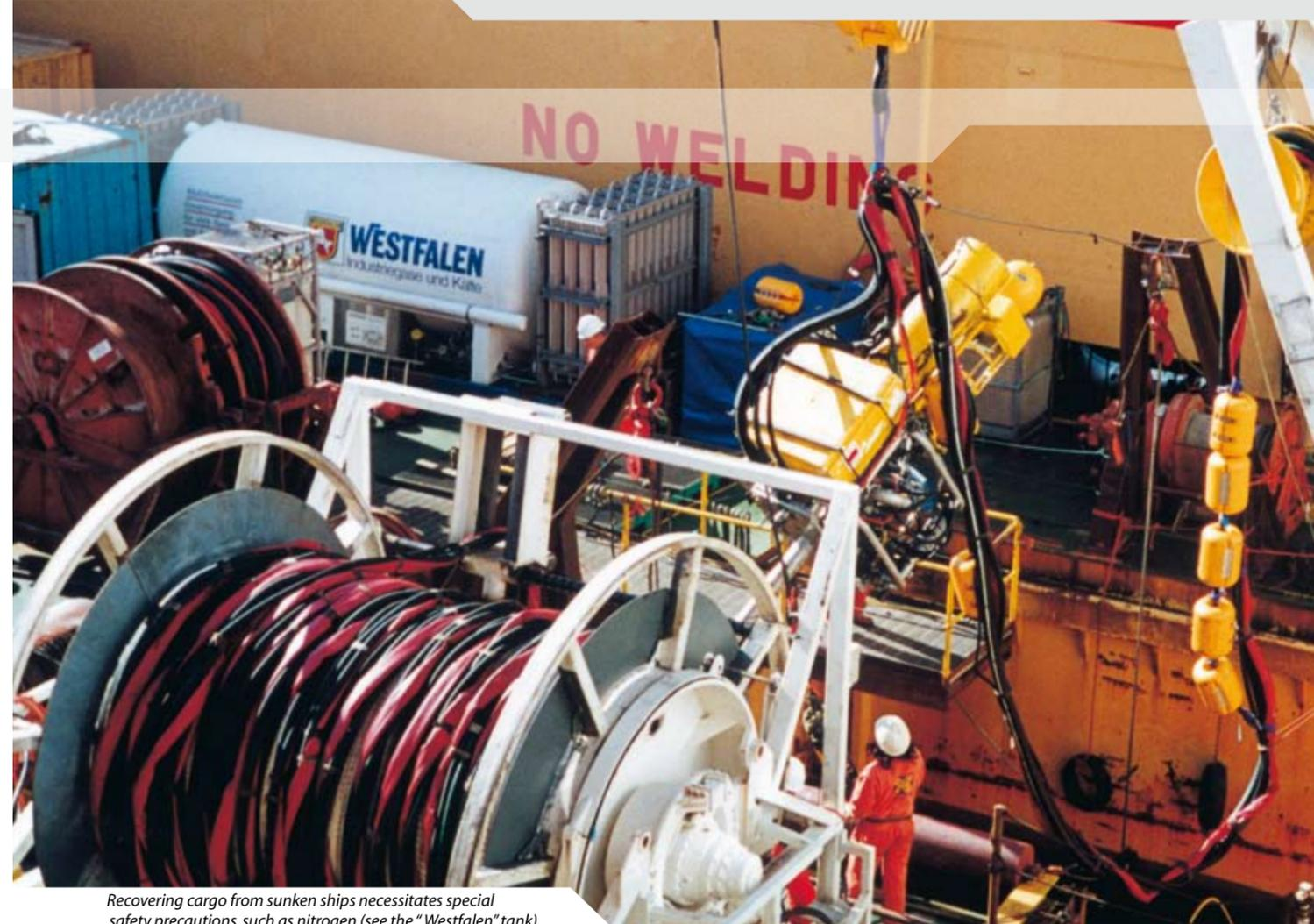
Recovering cargo from sunken ships necessitates special safety precautions, such as nitrogen (see the "Westfalen" tank).
