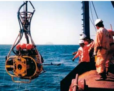
The first generation ROLS (Remote Offloading System), a component of the POLREC system.
