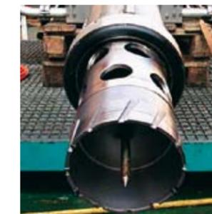
Close up of the 100 mm diameter "Double Bottom Tool". A central pin pushes the steel circle into the tank and the small reservoir in the mill collects the mill waste. Via the extended pipe the cargo will be pumped to the surface.
