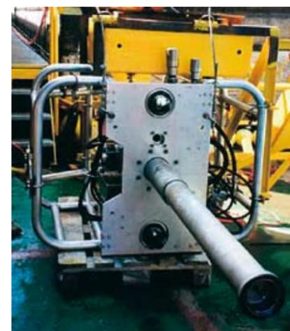
The "Double Bottom Tool" used for penetration of a double hull.
